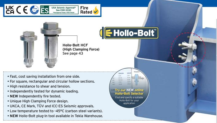
🜔 \* Carbon steel, hexagonal head Hollo-Bolts in all sizes have been independently fire tested in both tension and shear in accordance with ISO 834 and are fire rated up to 120 minutes. For further details and load data please contact Lindapter.
