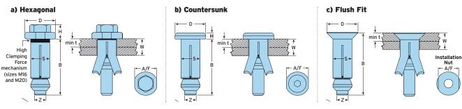
Material: Carbon steel or stainless steel (see page 41 for corrosion protection options)
