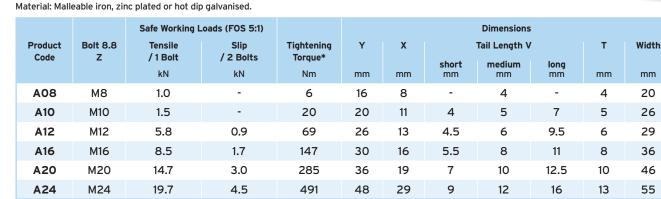
\* Torque figures based on bolts / setscrews in an unlubricated condition. For further information on lubricated fasteners see page 72.
